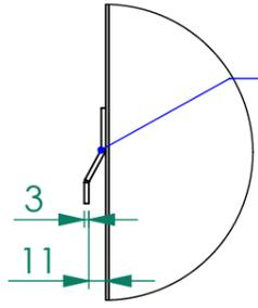
Brackets are fixed with M10 screws for boiler main shell
